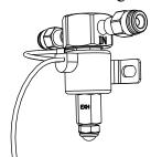
Use another straight fitting on the side marked "CYL" on the solenoid valve.
