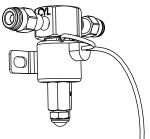
Connect an air line from the "CYL" end fitting to the union tee fitting. Connect an air line from the union tee to each of the chain units.(ref. Figure 3)
