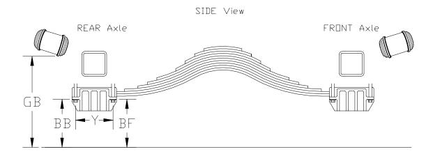
BF = Distance from ground to where capscrew flat washer contacts spring box in front
